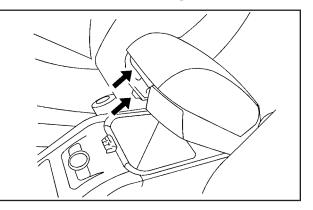
Your vehicle has a center console with an upper, lower and rear storage area. To access the upper storage area, lift up on the top lever. To access the lower storage area, lift up on the bottom lever. The top of the center console can extend forward. To adjust, hold the top of the lever up and pull the top of the center console forward.
